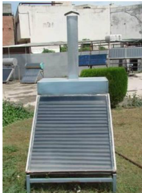
Figure 2-9 Solar Natural Dryer (Glazed Collector) 10-kilogram loading capacity PCRET
