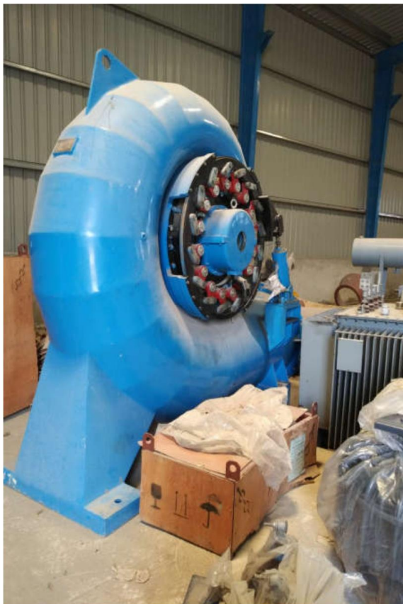
An imported Francis Turbine waiting to be installed (HEECO)
