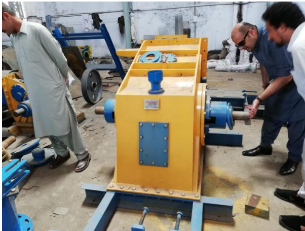
Figure 3-11: T-15 Crossflow Turbine Fabrication (Mukhtiar Engineering)
