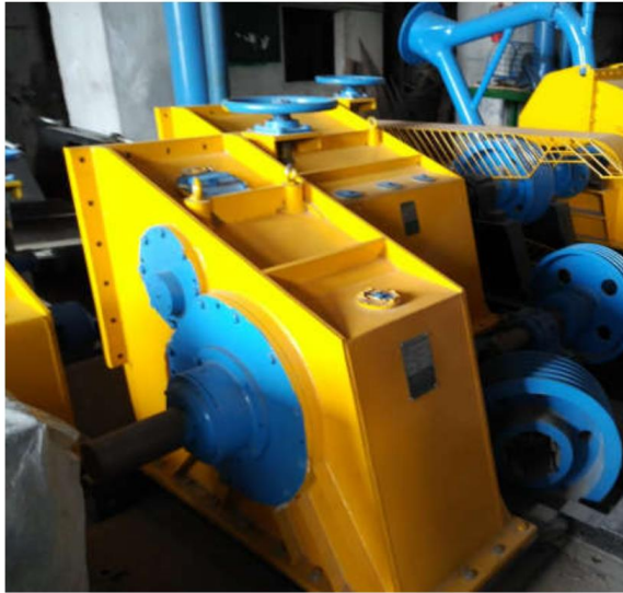
T-15 Crossflow Turbine manufacturing (HEECO)
