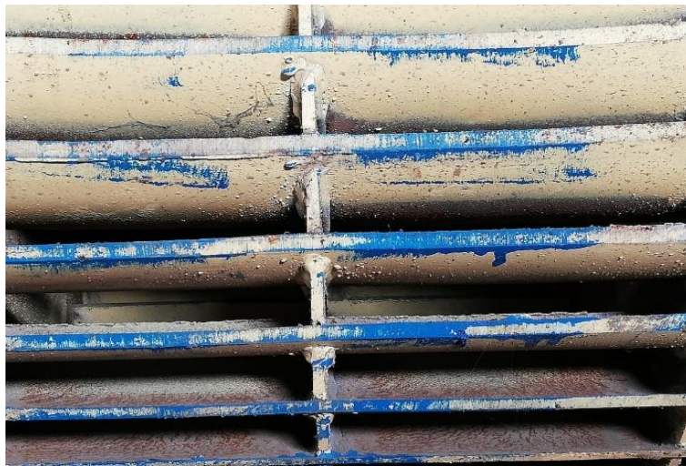
Figure 3-16: Defective Runner Blades (Rough Surface Finish)
