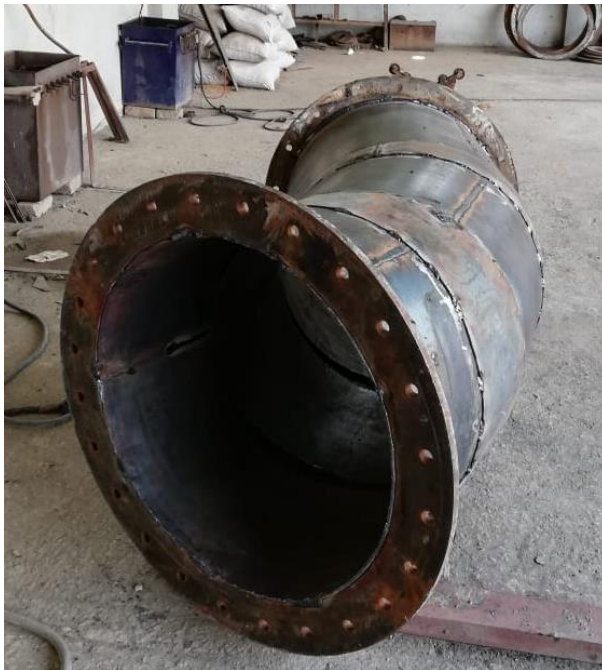
Figure 3-14: Penstock Fabrication (Mukhtiar Engineering)
